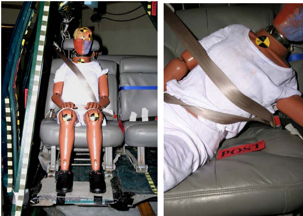
FIGURE 2: Pre- and Post-test belt positions for H3-5F (30 degrees)
