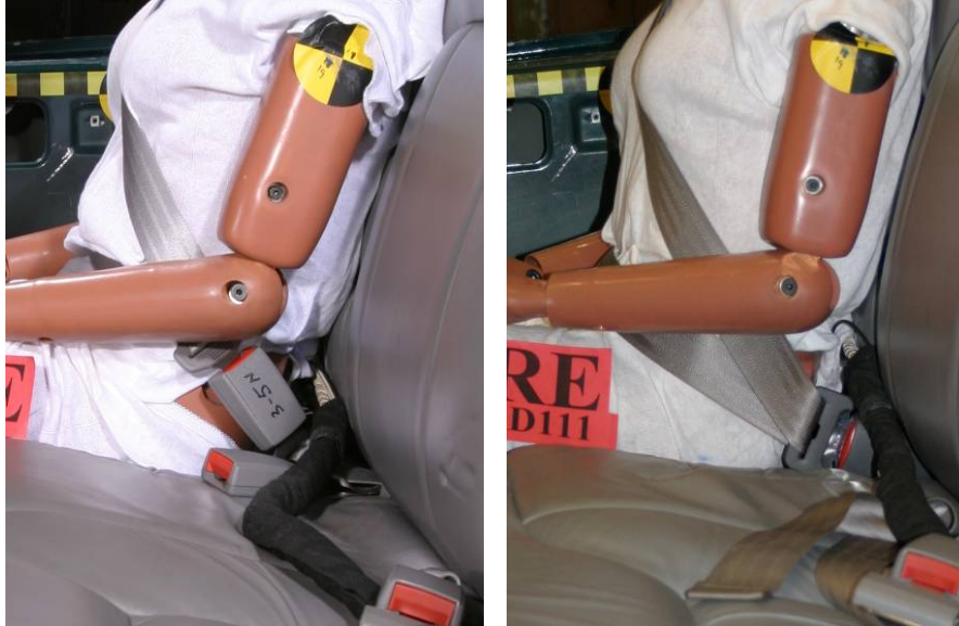
FIGURE 4: OEM Buckle (Allowed Submarining) vs. Modified Buckle Geometry (Prevented Submarining). The retro fitted buckle was attached solidly to the seat frame. The buckle could only be rotated a limited amount in the XZ plane.
